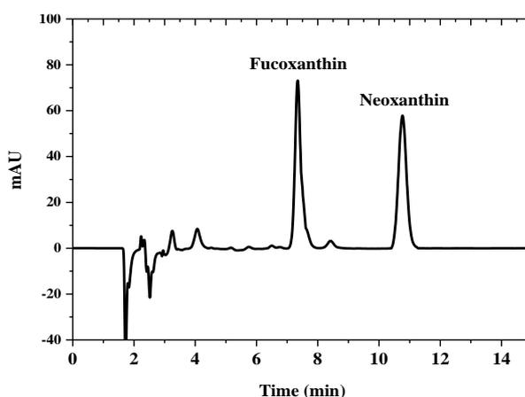
**Figure 2.** HPLC chromatogram for *Cylindrotheca closterium* extract (isocratic elution, 70:30-MeOH:ACN, column temperature: 25 °C, flow rate: 1.0 mL min<sup>-1</sup>, absorbance at 450 nm).
