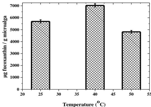
**Figure 5.** Effect of temperature on the extraction of fucoxanthin from *Cylindrotheca closterium* (Experimental conditions: 0.25 g microalga, 10.0 mL THF/DCM, 15 min sonication, n=3).
