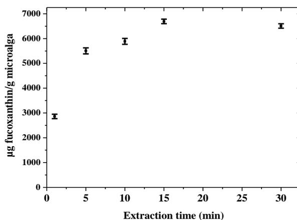
**Figure 3.** Effect of contact time on the extraction of fucoxanthin from *Cylindrotheca closterium* (Experimental conditions: 0.25 g microalga, 10.0 mL THF/DCM, 25 °C, n=3).
