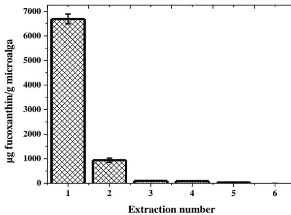
**Figure 4.** Effect of extraction number on extraction of fucoxanthin from *Cylindrotheca closterium* (Experimental conditions: 0.25g microalga, 10.0 mL THF/DCM, 15 min sonication, 25°C, n=3).
