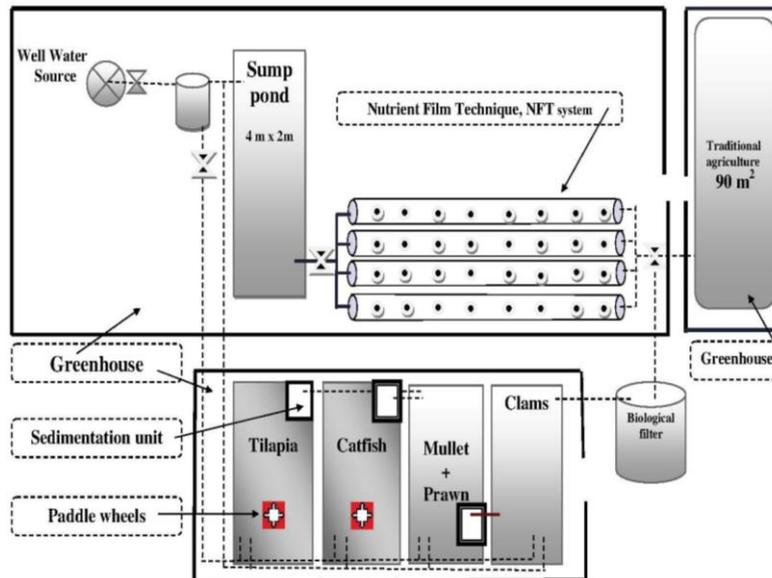
Figure 3. Schematic diagram of the IMTA-NFT.
