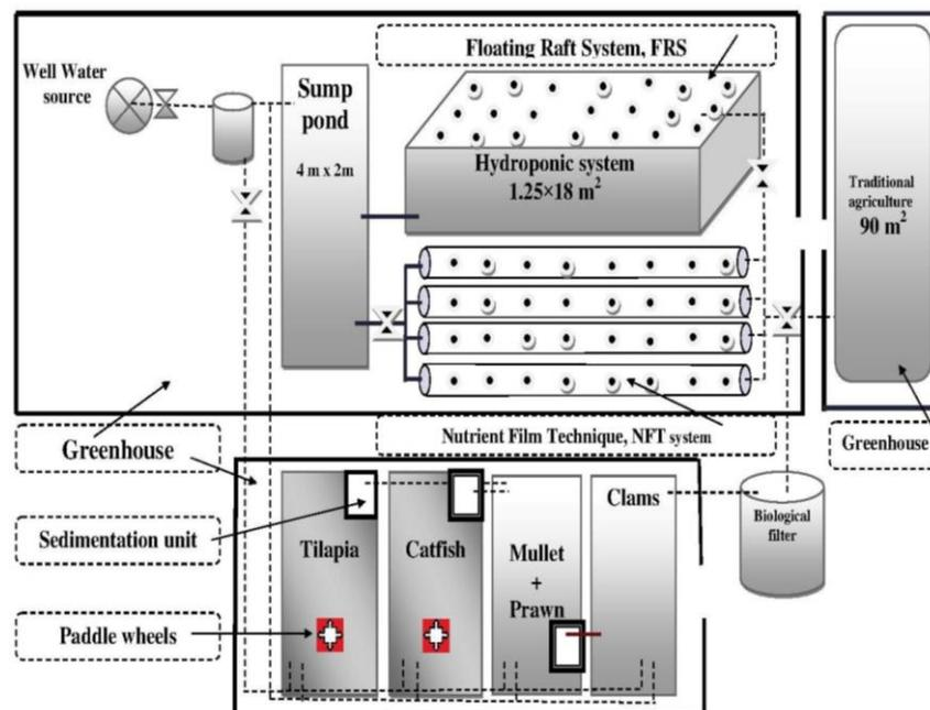
Figure 1. Schematic diagram of the IRAHS.
