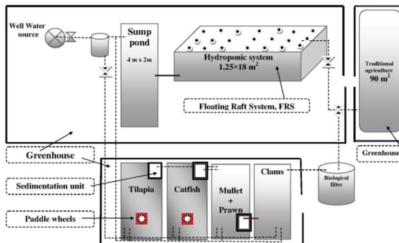
Figure 2. Schematic diagram of the IMTA-FRS.
