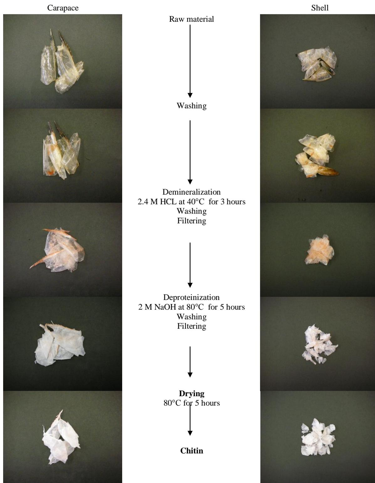
**Figure 1.** Overall process for the preparation of chitin from carapaces and shells.
