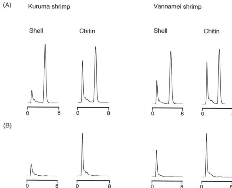
**Figure 3.** Typical chromatograms of oxolinic acid in shell and chitin, (A) shell and chitin samples spiked at 1.0  $\mu\text{g/g}$  oxolinic acid ; (B) control (without the drug).
