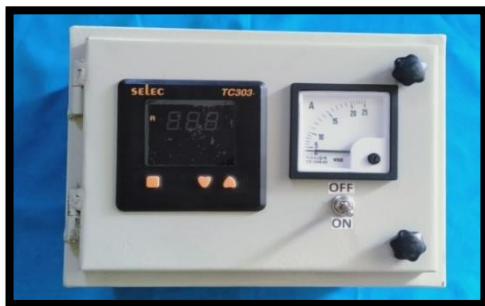
(F) PID Controller with Cut-Off System
