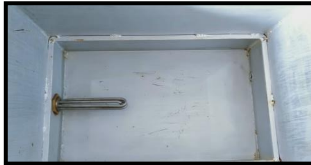
(E) Electrical Immersion Water Heater
