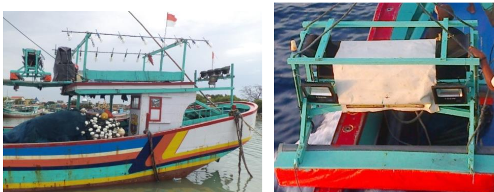
Figure 3. Fishing vessel with MH lamps (a) and bangkrak float with LED lamps (b).
