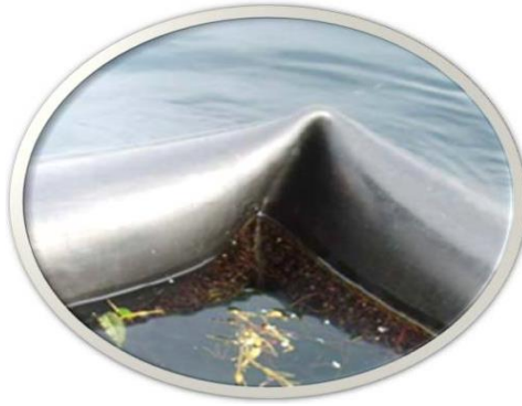
Figure 1. Common failure mode of the float collar for fish cage.
