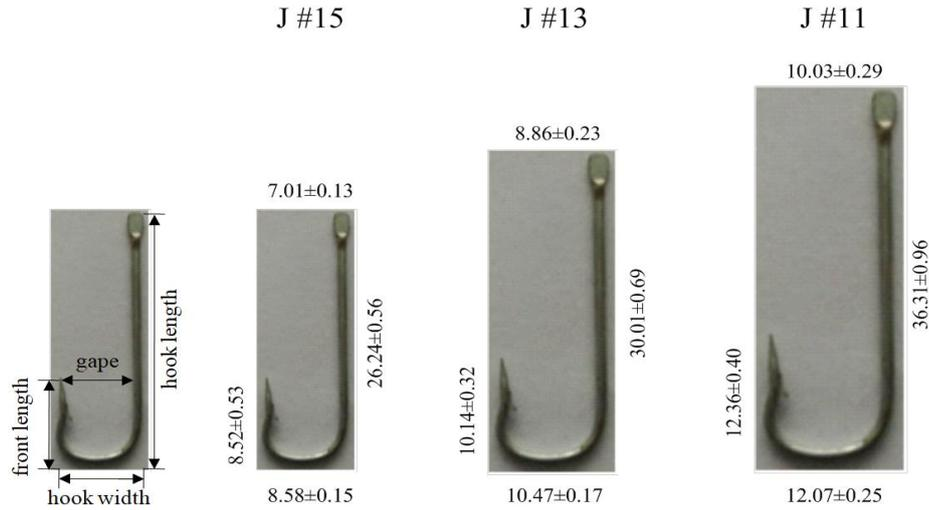
**Figure 2.** Shape and dimensions of three size hooks used in the selectivity study. Means and standard errors based on a sample size of 39 hooks for each type.
