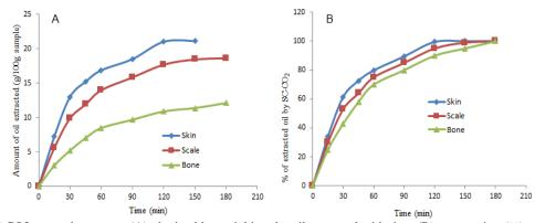
Figure 2. SC-CO2 extraction curves (A) obtained by weighing the oil extracted with time (B) progression (%) of oil extraction with time.
