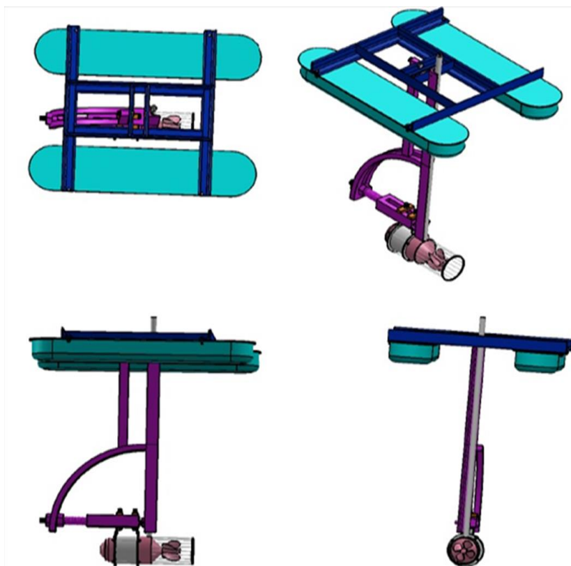
Figure 3. Different views of the modified aerator
