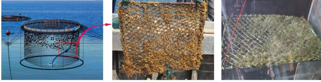
Figure 1. Images of the biofouled nettings of the net cage in fish farm.
