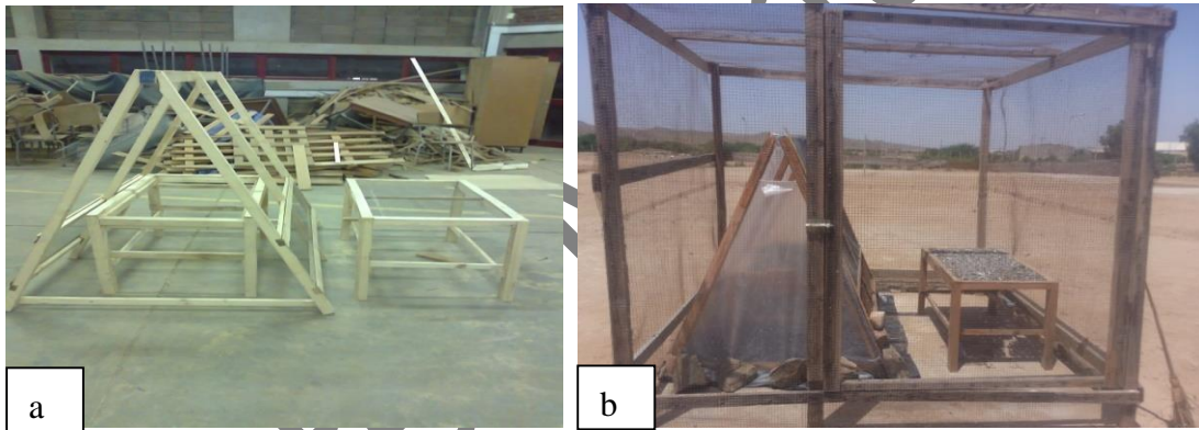
Figure 1. Construction of solar tent and open sun rack dryers (a) and drying of studied fish (b)
