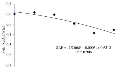
Figure 5. Variation of SAE with different submersible depth (d) of the propeller shaft.
