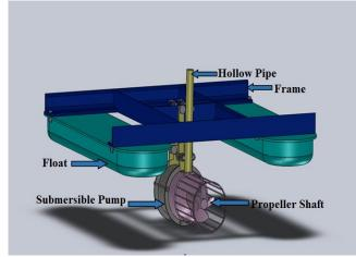
Figure 1. A view of submersible aerator before modification.
