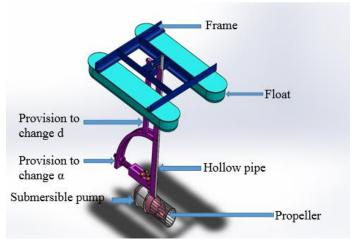
Figure 2. A view of submersible aerator after modification.
