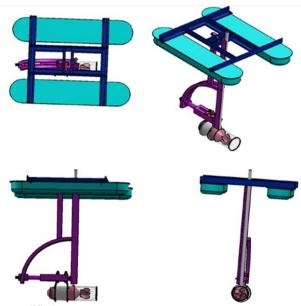
Figure 3. Different views of the modified aerator.
